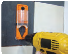
Place tip of drill bit into the guide position. Then start drilling.
